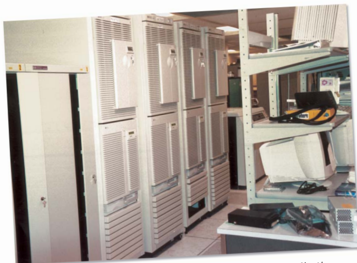
A variety of HP3000s, HP9000s and smaller servers host applications such as PeopleSoft, AMANDA, iRIMS and the GNWT e-mail system. The servers are available to GNWT staff 24/7/365, except for backup time after midnight.
