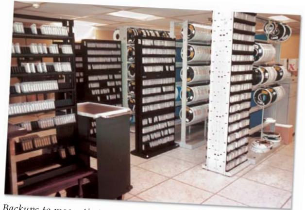
Backups to magnetic tape are critical. Computer Operators do the backups regularly, ensuring that any data from any computer system can be recovered if required, in case of server or application malfunctions. About 8,000 magnetic tapes are used for the backups. The majority of these tapes are kept off site in secure storage, ensuring data remains available in case of serious damage to a data centre.
